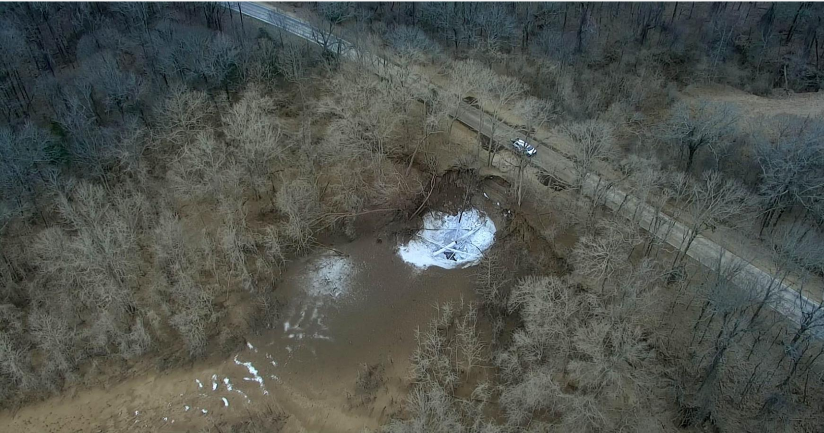
A 24-inch pipe rupture in Yazoo County, Miss. occurred on Feb. 23, 2020
