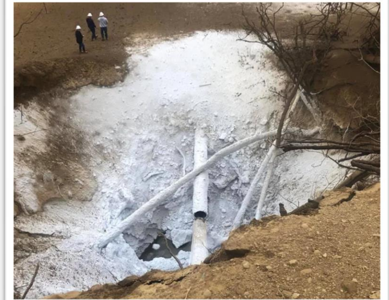
A 24-inch pipe rupture in Yazoo County, Miss. occurred on Feb. 23, 2020
